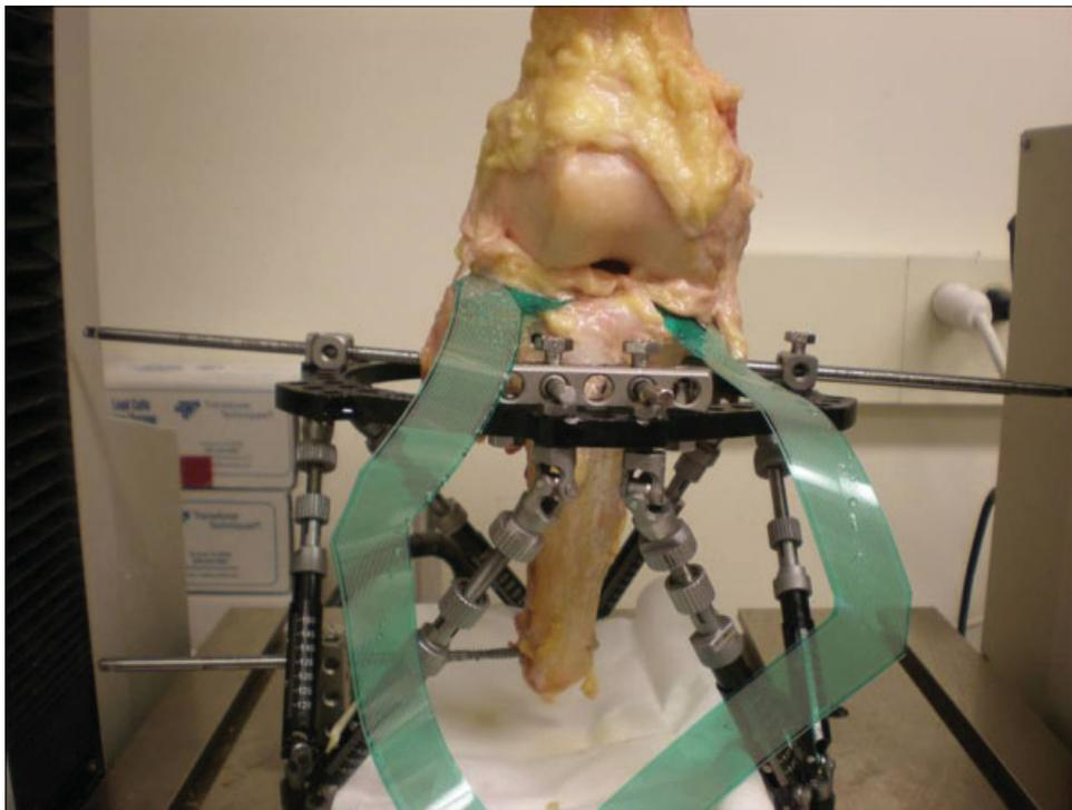
**Figure 1** Testing setup. Tibia in Taylor Spatial Frame with femur in MTS machine and Tekscan sensors placed submeniscally. Real-time pressure measurements were collected in the medial and lateral compartments.
