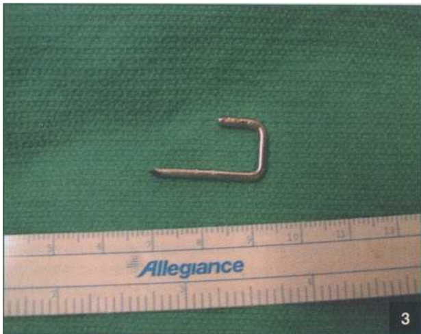
Figure 3. Photograph of removed staple. One arm broken, the other intact, implicating pullout and fatigue failure.
